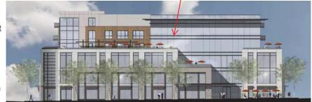
2. Add a projecting cornice or roof canopy at the second level to emphasize the two-story massing along street frontages to better relate to the adjacent new projects and the pedestrian scale of the sidewalks. At the planning commission's discretion, the third floor could also be setback to reduce its impact on the overall building massing and the human scale of adjacent pedestrians.
