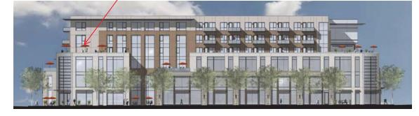
**Response**: The design uses both vertical and horizontal articulation and layering to break up the massing of the 6-story building.
